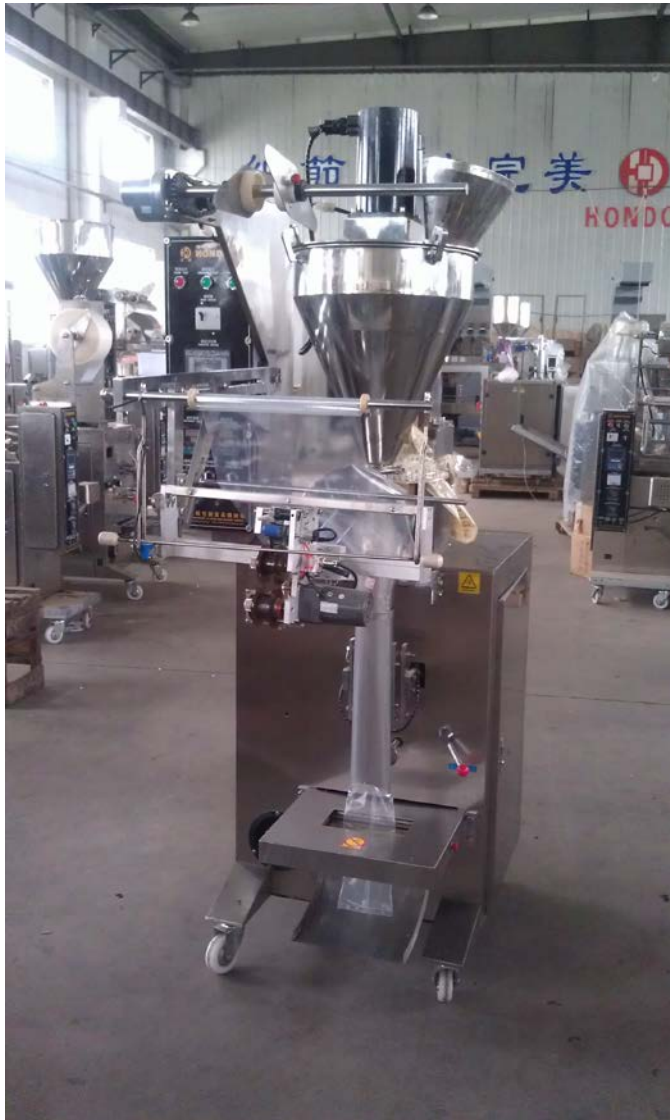
DXDF-800 automatic powder packaging machine
